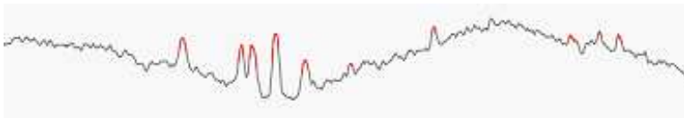
Figure 3: Effect of the adaptive thresholding method on a single intensity profile. Resulting foreground segments are marked red.
