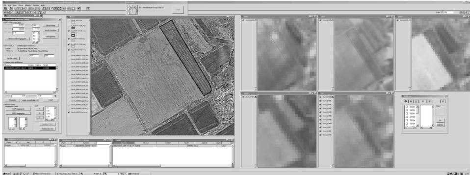
Figure 4: A screenshot of the Computer-Aided Photo-Interpretation software. (Large window on the left: VHR image, small windows: HR image time series)
