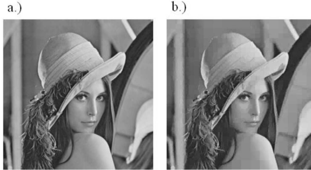
Figure 1: Original (a) and decoded (b) test images of Lena 256 \times 256 using the proposed classification encoding method at compression ratio 1.4 bpp and with reconstruction fidelity PSNR=31.60
