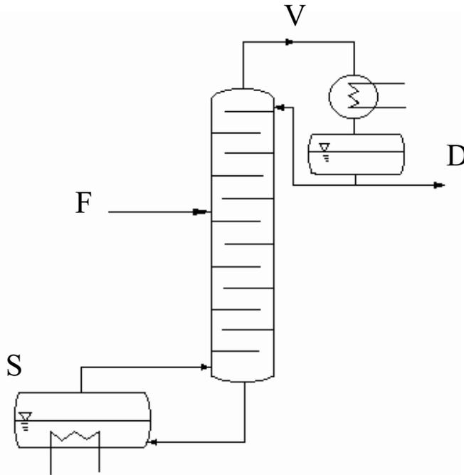
Figure 1: Batch extractive distillation process
